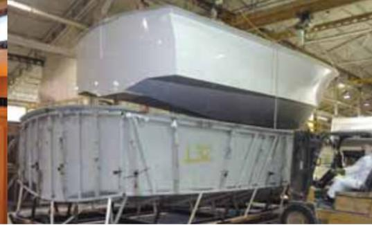
Legacy powerboats are built right alongside Tartan sailboats in the manufacturer's Fairport Harbor, Ohio, factory. Here, a Legacy 32 hull is being pulled from the mold.
